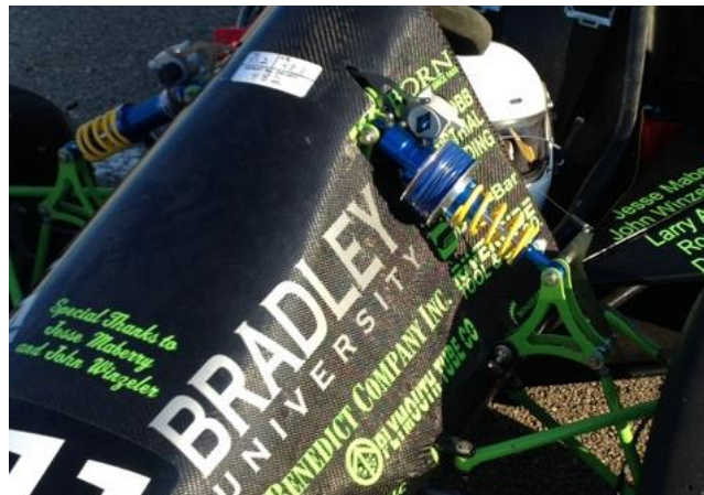
Figure 36: MR Damper Installed on a Formula SAE Car
