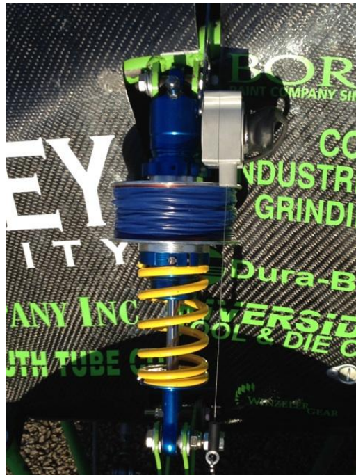
Figure 24: MR Damper Installed on Formula SAE Car
